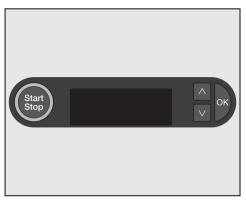
The display is operated using the  $\land$ ,  $\lor$  and **OK** buttons.
